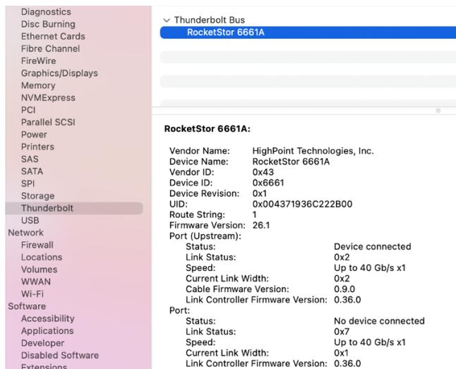
If the RocketStor 6661A entry is not displayed, this may be related to a connection problem – move the RS6661A to another Thunderbolt™ 3 port or replace the cable and recheck the entry.
