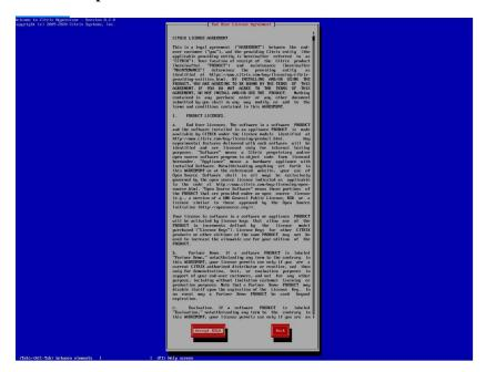
6. After confirming the EULA agreement, you will be asked to select the target disk. Select the RAID array as the target disk to install the Citrix Hypervisor 8.2. You can then proceed normally - follow the onscreen prompts to install Hypervisor to the array.
