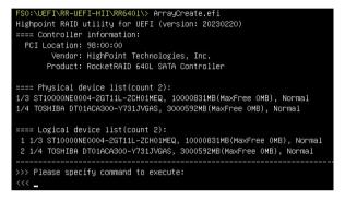
d. Command "create RAID0". Create RAID0 array with all disks and with maximum capacity.
