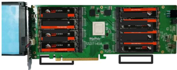
步骤 8. After installing all SSDs, carefully flip the heatsink to the right.
