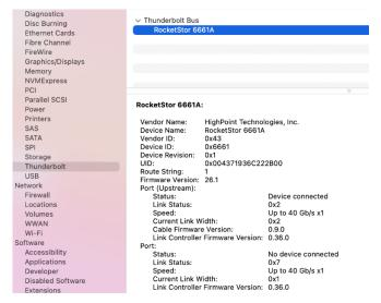
If the RocketStor 6661A entry is not displayed, this may be related to a connection problem – move the RS6661A to another Thunderbolt<sup>TM</sup> 3 port or replace the cable and recheck the entry.
