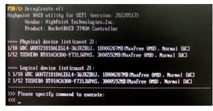
e. Command "create RAID1". Create RAID1 array with all disks and with maximum capacity.
