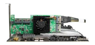
Connect the remaining NVMe SSDs to the SSD7580A controller as described above. Once complete, Power on the system
