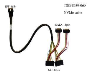
2. Shown above is a SFF-8654 to U.2 SFF-8639 cable with a 15-pin SATA power connector. The SFF-8639 port should be connected to the NVMe SSD's U.2 port. The 15 pin SATA power connector should be connected to the system's power supply.
