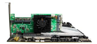
As described in step 2, connect the SFF-8639 cable connectors to the U.2 SSDs. Next, connect the SFF-8654 cable connector to one of the SSD7580B's four device ports (Ports 1 through 4).
