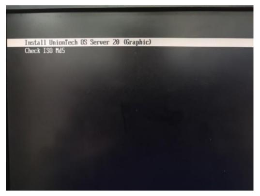
When the installation switches to the graphical installation, press "Ctrl+ALT+F2" to switch the shell on console 2 before select "Next".
